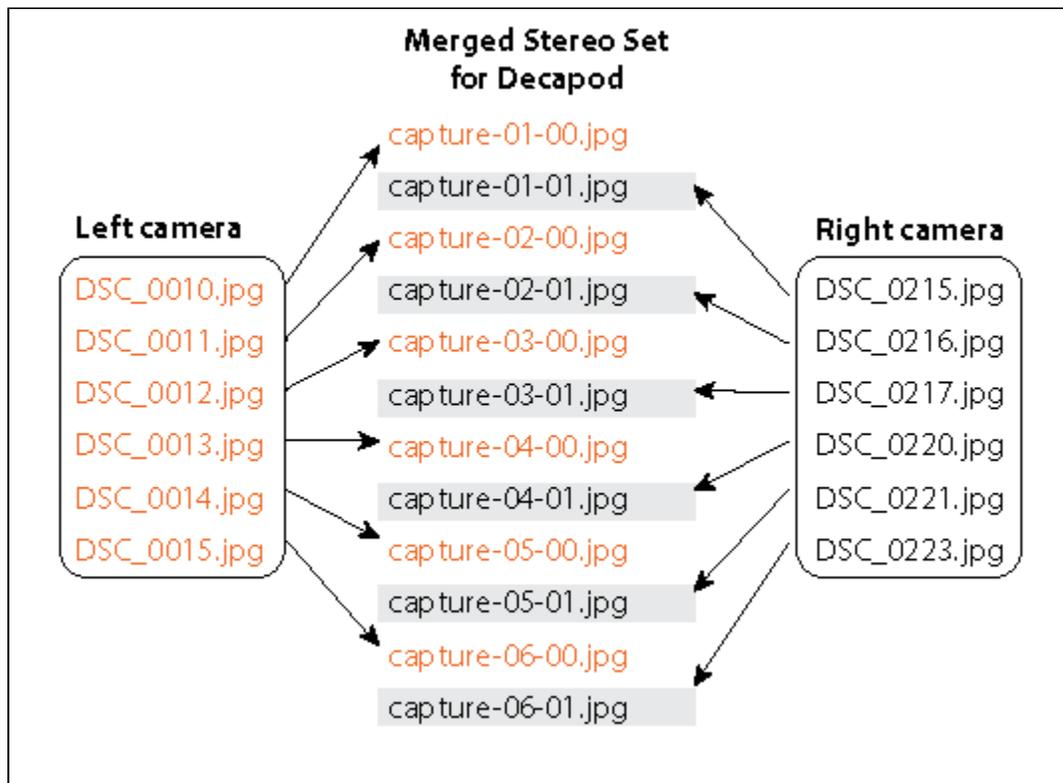
In this example, files from left and right cameras are renamed to create matched pairs. Files with "-0" are for the left images, and "-1" are for the right images.
